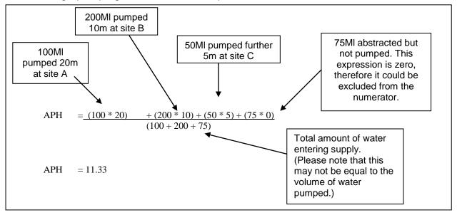
The average pumping head should be calculated using data from all sites if possible. SW should state in its commentary if sites have not been used in calculating the average pumping head, and why they could not be used.
